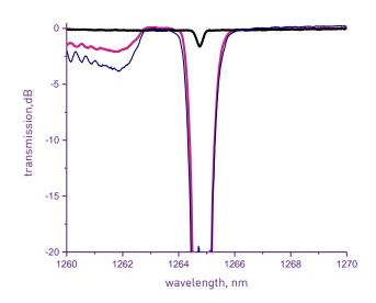
0.7nm. Output grating with reflectivity 5% - 40% has FWHM 0.15 – 0.35nm. Mismatching LR grating relative to HR one is up to  $\pm$  0.1nm. For fiber lasers with narrow line we are presented FBG pairs with FWHM around or less 0.1nm with ideal matching without adjustment. The transmission spectrum of FBGs Pair for Yb laser and Raman converter are presented in the graph.
