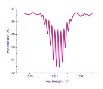
alow-finess Fabry-Perot cavity. The transmission spectrum of Fabry-Perot fiber interferometer is presented in the graph.
